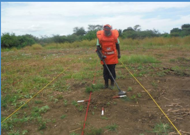
A deminer used a metal detector to detect potential explosive hazards for removal and destruction in Mogiri, Central Equatoria.
